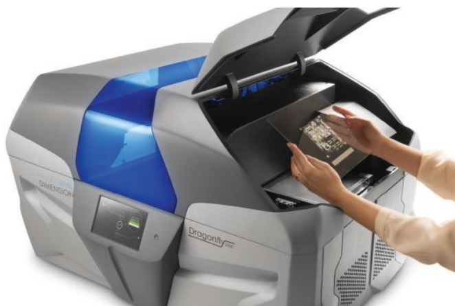
The Nano Dimension dual-material inkjet Dragonfly 2020 3D printer creates professional multi-layer printed circuit boards that include vias, without the need for drilling. The equipment deposits both dielectric and conductive inks and performs an integrated sintering process for curing both materials. Image courtesy of Nano Dimension.
