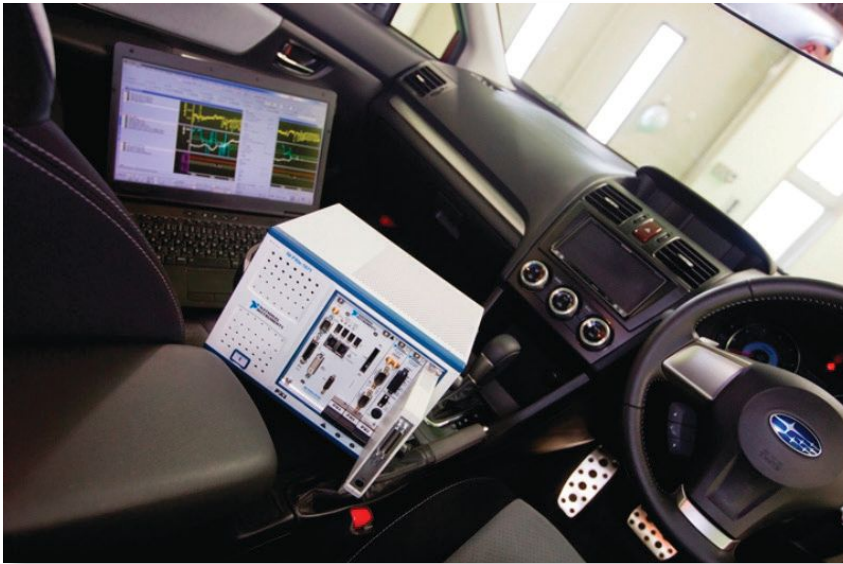
National Instruments' hardware-in-the-loop technology combines physical testing and simulation to ensure that systems will behave as expected prior to actual field testing. Image courtesy of National Instruments.
